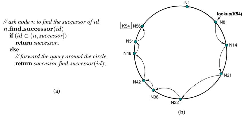
Fig. 3. (a) Simple (but slow) pseudocode to find the successor node of an identifier  $id$ . Remote procedure calls and variable lookups are preceded by the remote node. (b) The path taken by a query from node 8 for key 54, using the pseudocode in Figure 3(a).
