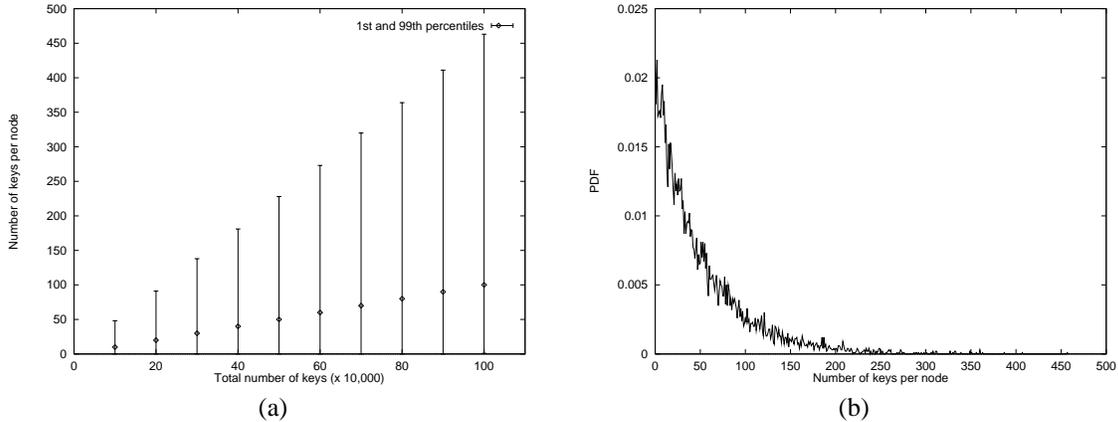
Fig. 8. (a) The mean and 1st and 99th percentiles of the number of keys stored per node in a  $10^4$  node network. (b) The probability density function (PDF) of the number of keys per node. The total number of keys is  $5 \times 10^5$ .
