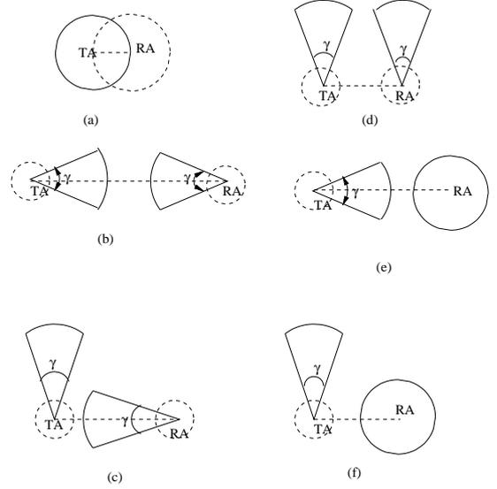
Figure 1: Relevant configurations between transmitting antenna (TA) and receiving antenna (RA), depending on the antenna type. Figure (a) corresponds to a pair of OAs. Figures (b), (c), and (d) illustrates the relevant configurations for a pair of DAs. The mixed case, i.e., the configurations corresponding to OA and DA are illustrated in figures (e) and (f). Notice that if the TA becomes RA and vice versa, the communication range remains the same.
